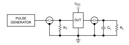
$C_L=50$  pF at  $V_{CC}=3.3\pm0.3$  V or equivalent (includes jig and probe capacitance)  $C_L=30$  pF at  $V_{CC}=2.5\pm0.2$  V or equivalent (includes jig and probe capacitance)  $R_L=R_1=500~\Omega$  or equivalent  $R_T=Z_{OUT}$  of pulse generator (typically  $50~\Omega)$
